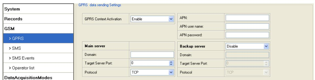
Figure 15 GPRS configuration
